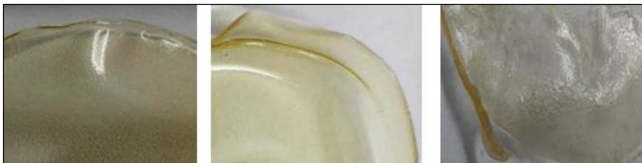
Fig 1: (a) Physically crosslinked; (b) Chemically crosslinked; (c) Double crosslinked hydrogels
